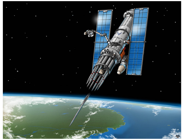
Figure 4. Artist's impression of a kinetic bombardment device. The rods being launched are solid rods composed of tungsten. 21
